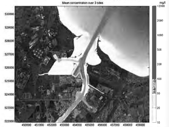
Figure 5-2 Simulated sediment release from TSHD dredging in spring tide, low river flow conditions a) average increase in suspended sediment concentration b) deposition after 3 tides of dredging
